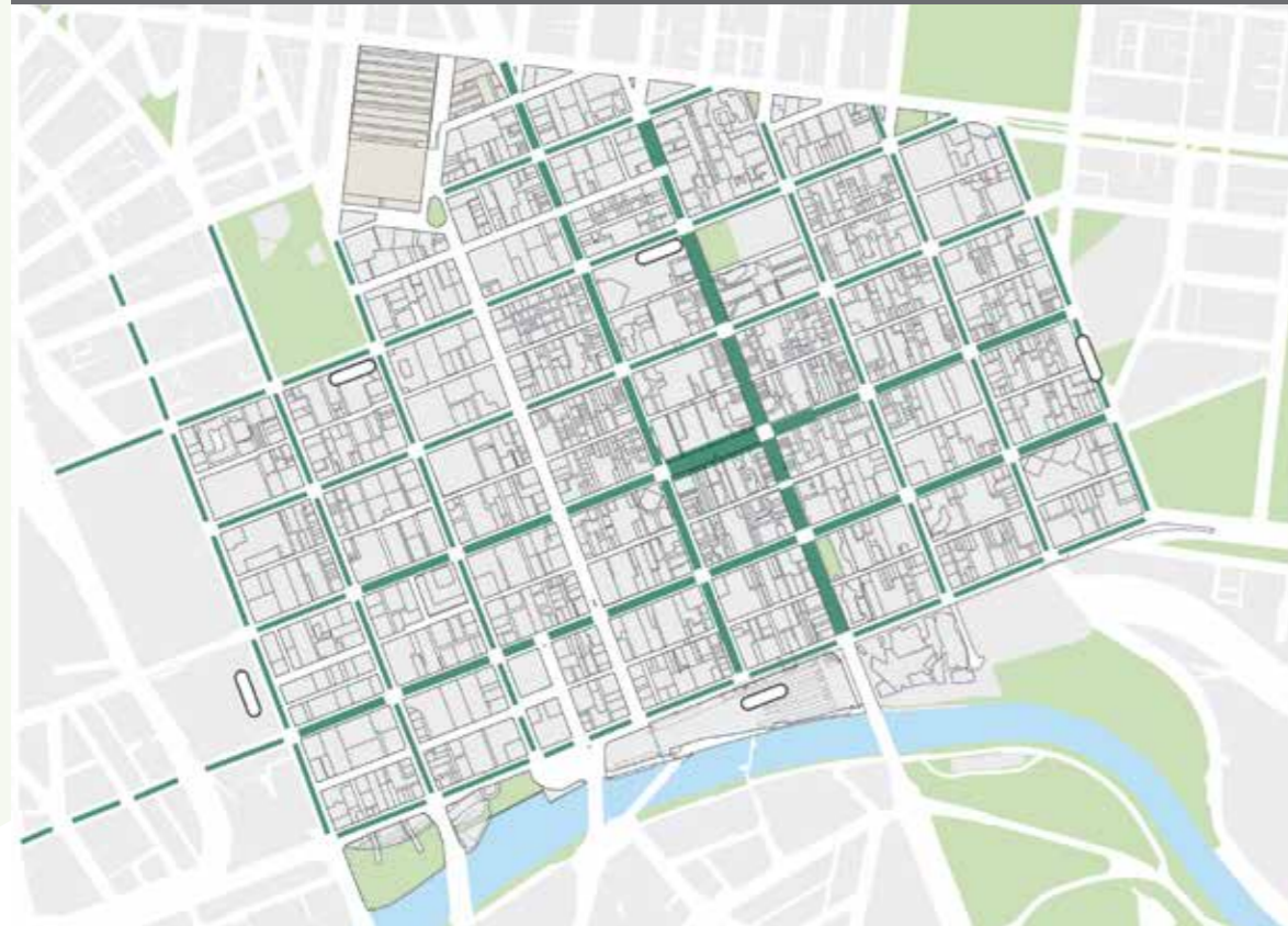
Map indicating footpath widths ranging from narrow (-3.6 m) to moderate (-5.4 m) to wide (-8.5 m).
