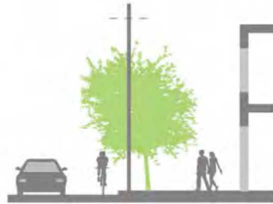
Small tree under powerlines
