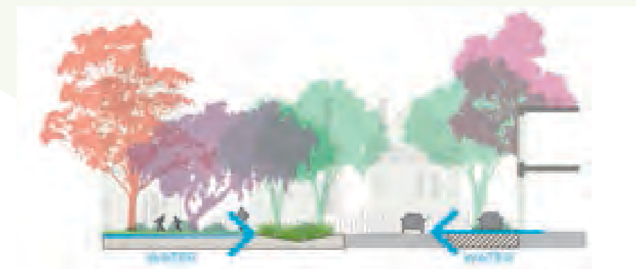
Water infiltration, permeable paving and structural soil or cells provide opportunities to grow larger, healthier trees in paved areas.
