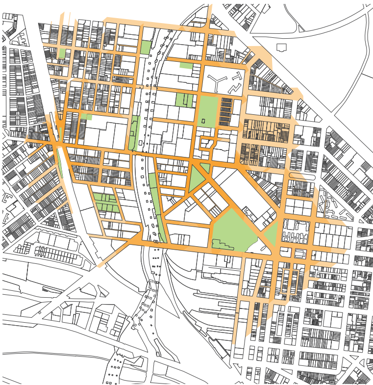
Figure 5.8: Proposed Condition - Extent of pedestrian access to open space (according to park type)
