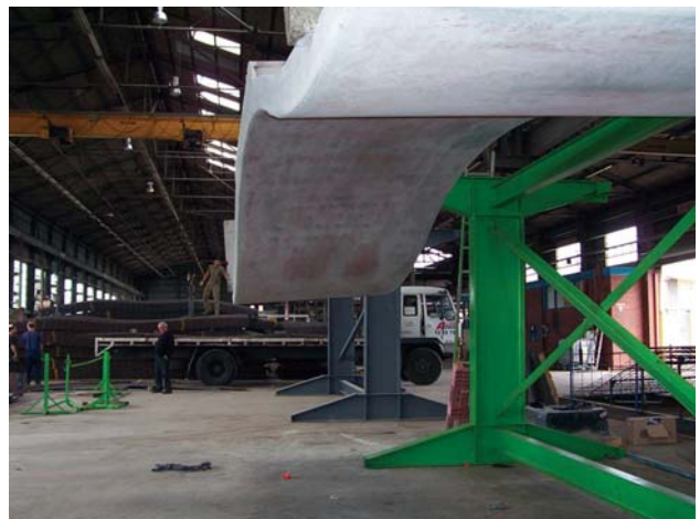
F. Finished undulating ceiling panel.
