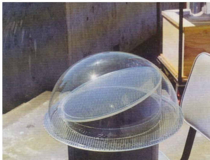
Figure 10: A tilted laser cut light-deflecting panel
