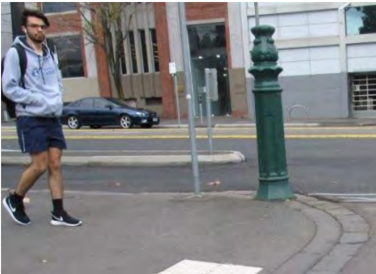
Figure 19: Swanston Street Carlton – Five row wide pitcher channel in side street intersection reduced to a single row to accommodate access ramps
