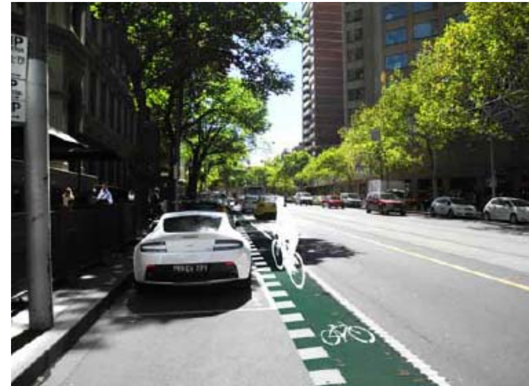
Investigate the provision of innovative bicycle facilities to address car dooring crashes, using green surfaces, buffer zones and vibra-lines.
