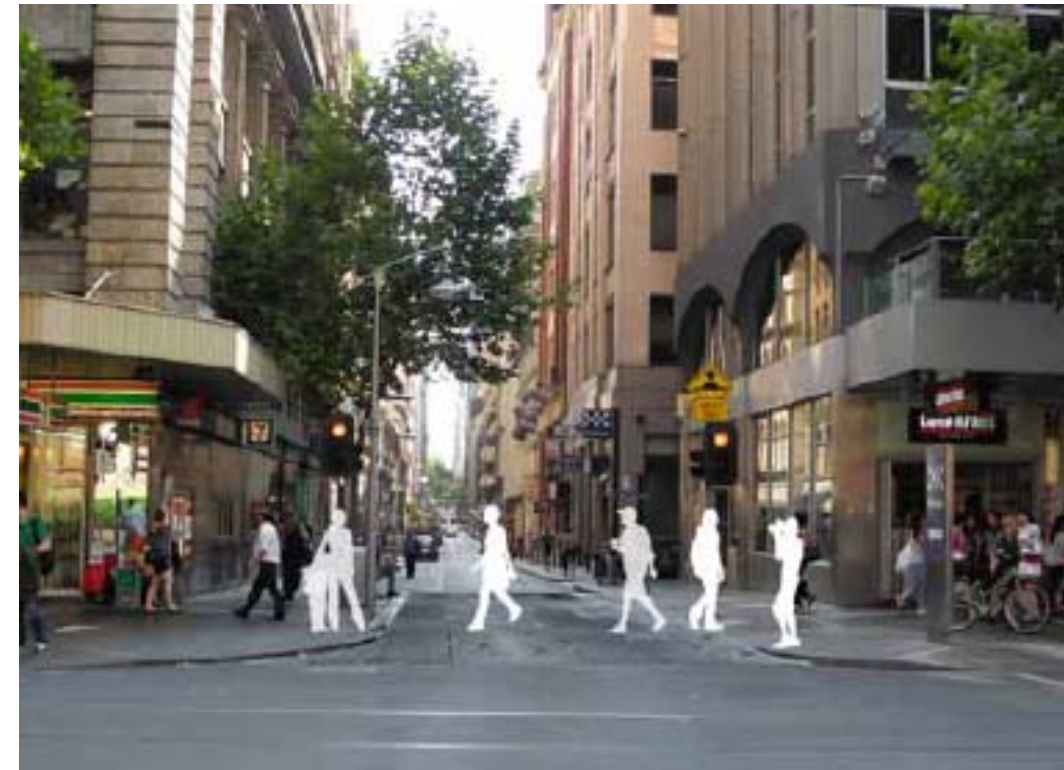
Remove footpath interruptions by raising the roadway for level access at suitable locations.
