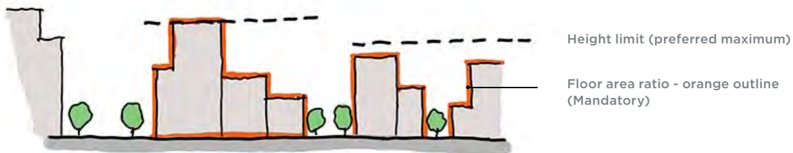
Figure 2.2: Floor area ratios help to control the density, or intensity, of the development in relation to the size of a site. The orange outline above highlights a potential allowed density of a site according to a floor area ratio control. When used in combination with design objectives such as setbacks, floor area ratios can enable a better response to the surrounding context and character of a site, allowing for a greater diversity of buildings while placing a natural cap on height.
