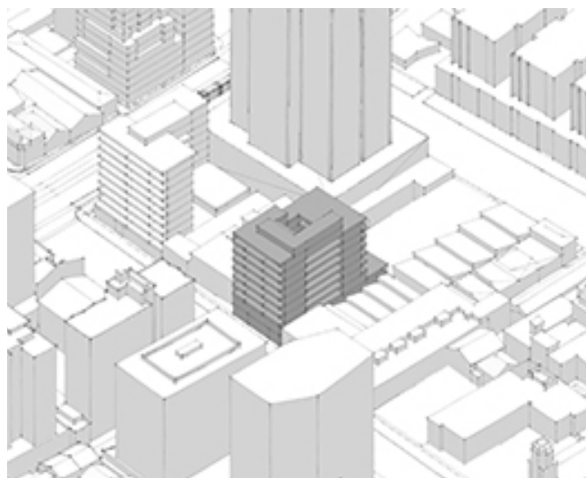
Figure 3.16: Built form testing to show the proposed floor area ratio and built form controls on a mid-block site in Flagstaff (DDO33). Images are indicative only to test the proposed controls and are not representative of actual building proposals (West Melbourne Built Form Testing, Breathe Architecture).
