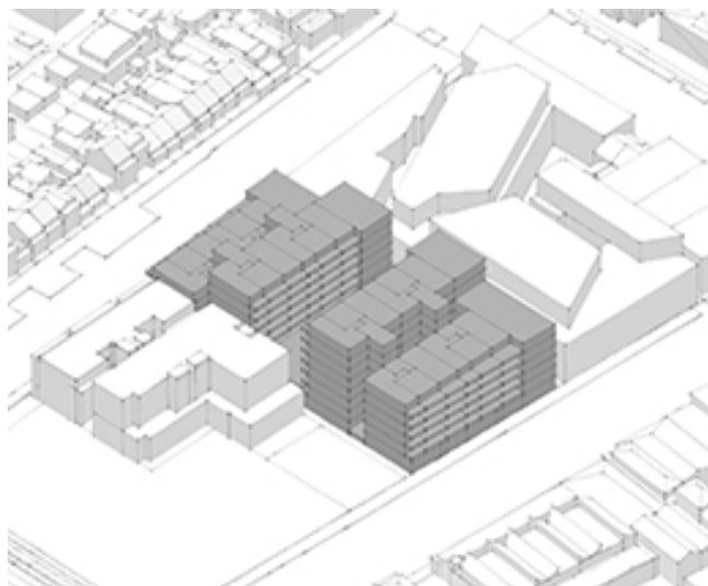
Figure 3.7: Built form testing to show the proposed floor area ratio and built form controls on a mid-block site in Spencer. Images are indicative only to test the proposed controls and are not representative of actual building proposals ( West Melbourne Built Form Testing , Breathe Architecture).
