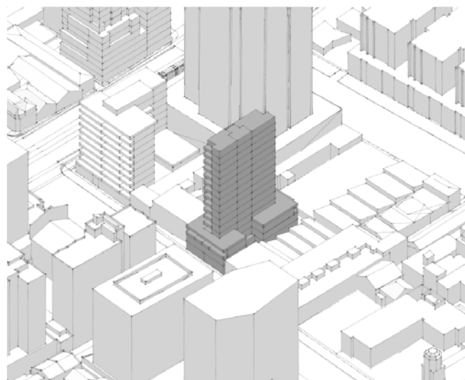
Figure 3.17: Built form testing to show the proposed floor area ratio and built form controls on the same mid-block site in Flagstaff (DDO 33), offering a different typology. Images are indicative only to test the proposed controls and are not representative of actual building proposals (West Melbourne Built Form Testing, Breathe Architecture).
