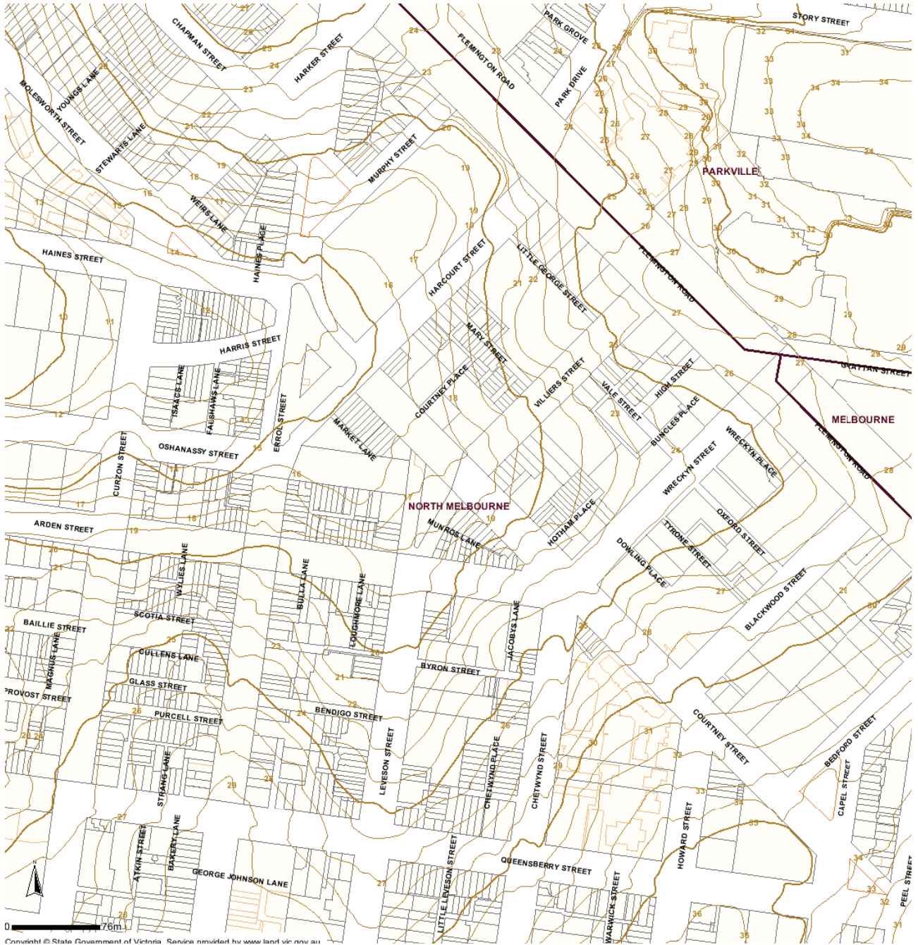
Contour map showing Errol St and Courtney St intersection is lower than Arden St by about 5m.
