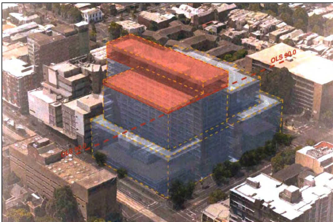
DPO potential building mass and encroachment into Operational Airspace - Source: Applicant documentation
