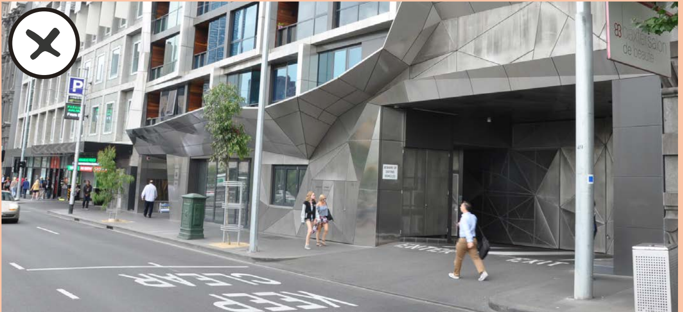
The positioning of vehicle access, loading and services on main street frontages.
