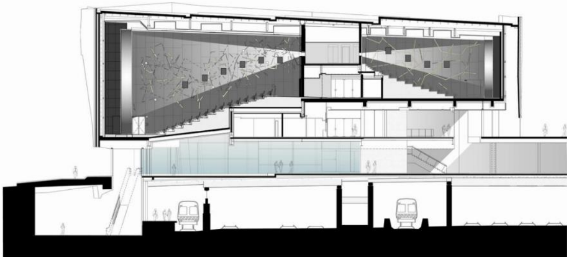
Section through ACMI cinemas down through decking to rail line below. Source: LAB Architecture Studio
