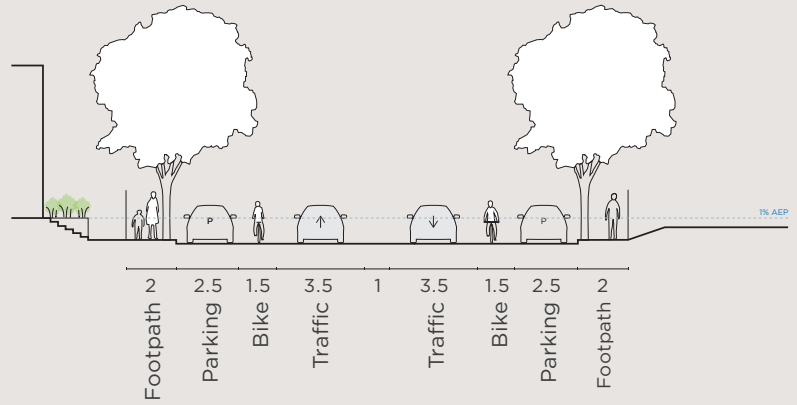
Figure 1.37: Existing street sections
